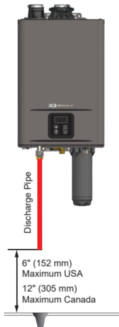
Figure 38 - Discharge Pipe Clearance
