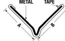
Award Metals SUN LINE™ trims are produced to meet ASTM C-1047 except for Section 4.1.
