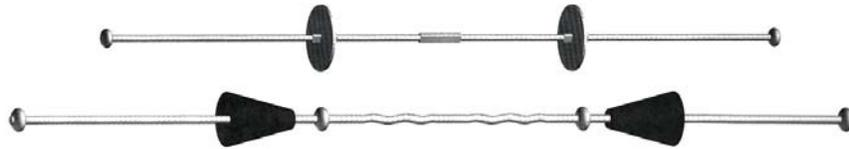
*Note: 2250 lbs. allowable with 2.0 safety factor, short end or long end. Rap-I-Form® Metal Washer and Plastic Cone Snap Ties are now available in wall sizes 6" through 24".*
