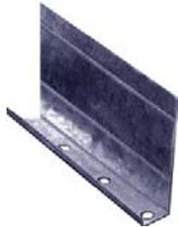
**Award J-8 Drip Mold Metal** is generally used as plaster or stucco stop at the mud sill. Manufactured with 3½” wall flange to meet current codes. The 7/8” base is available with or without weep holes.
