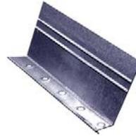
**Award #36L Stucco Stop** is generally used for exterior 3 coat stucco wall applications. Manufactured with a full 3½” wall flange to meet current codes. The wall flange also has 2 stiffeners that can be used to align stucco stop for 13/16” or 5/16” coverage at the mud sill. Available in 7/8” ground only. Available with weep holes.
