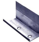
**Award J-33 One Coat Screed** is generally used with foam board for one coat stucco applications. Manufactured with a full 3½” wall flange to meet current codes. The 1¾” base is available with or without weep holes.
