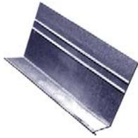
**Award #34L Stucco Stop** is generally used for exterior 3 coat stucco wall applications. Manufactured with a full 3½” wall flange to meet current codes. The wall flange also has 2 stiffeners that can be used to align stucco stop for 13/16” or 5/16” coverage at the mud sill. Available in 7/8” ground only.
