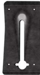
Award Rap-I-Form® Flat Snpatie Wedge is used to take up and secure flat snaptie ties to the panels. The wedge is secured with a vertical hammer blow and is released during stripping with a reverse hammer action.
