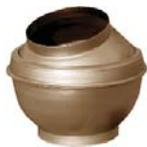
Spun steel galvanized ball joints provide flexibility in ducts serving moving cutter heads or other moving equipment. Thus, duct can swing through on arc while maintaining exhaust flow in the line.
