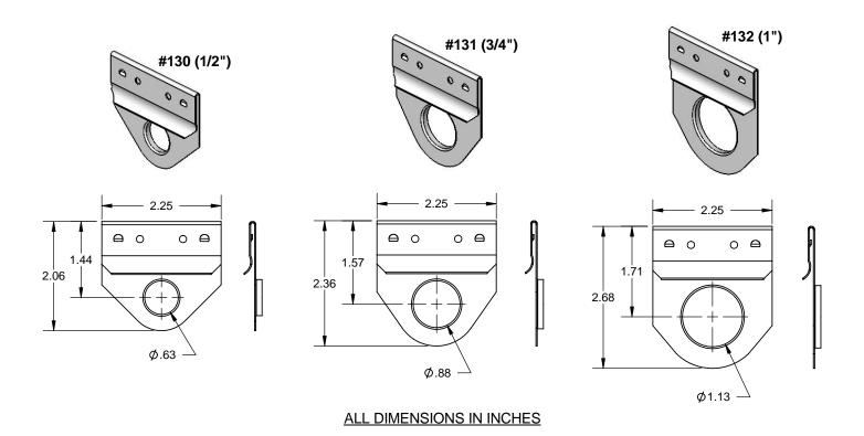
The HOLDRITE<sup>®</sup> #130, #131, and #132 are Solid Copper clips. Designed for easy snap-on installation for various flat strap brackets.  $\frac{1}{2}$ ",  $\frac{3}{4}$ " or 1" copper tubes solder directly to the clip.
