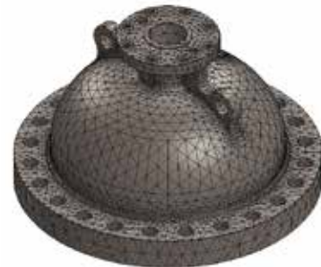
FINITE ELEMENT MESH USED IN OPTIMIZATION STUDIES
