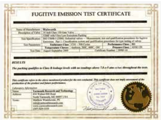
Emissions after 500 cycles at ambient and 350 °F Issued by Yarmouth Research and Technology Lab for 16 inch Class 150 Gate Valve After 500 cycles the measurement result was less than 50 ppm.
