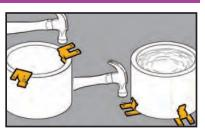
Pipe Sleeve Fasteners
