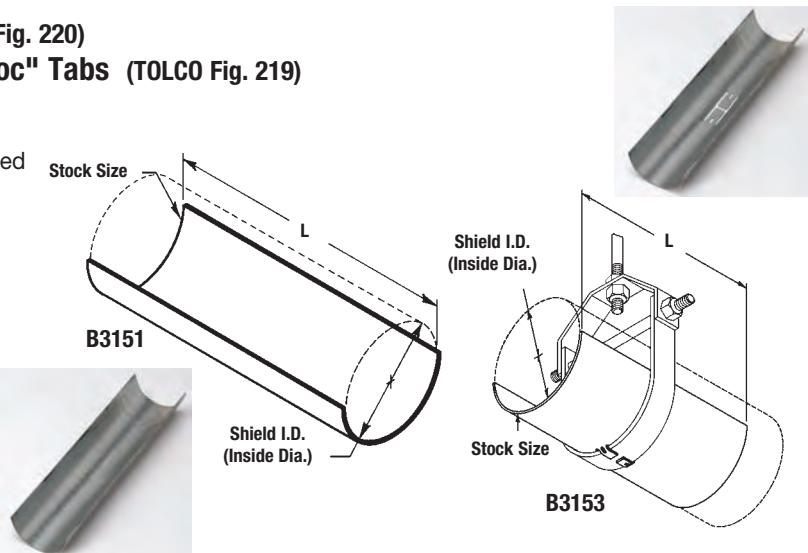
B3153 same dimension as B3151, but with bottom tabs for centering and securing the shield to hanger.
