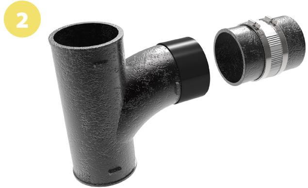
Place Neoprene® gasket on no hub cast iron pipe or fitting, firmly seated against the raised stop mark of pipe or fitting. Place stainless steel shield assembly over the end of other pipe.
