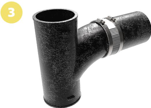
Butt ends of no hub cast iron pipe or fitting together inside the gasket until both are firmly seated against the center stop of gasket. Center the stainless steel shield assembly over the gasket.
