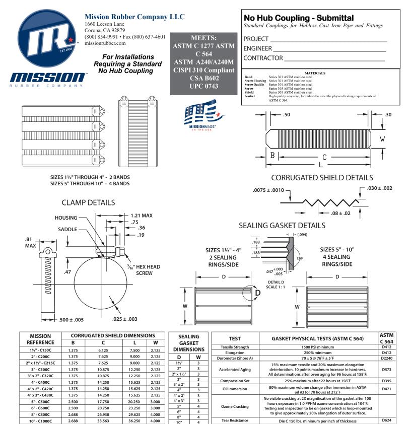
**Mission's No Hub Coupling** is designed to connect cast iron hubless soil pipe and fittings in sanitary and drain waste and vent (DWV) applications. Couplings consist of two (2) or four (4) 301 series stainless steel clamps attached to a 301 series stainless steel corrugated shield, over a molded one-piece elastomeric sealing gasket. Couplings are available in sizes  $1\frac{1}{2}$ " to 10":  $1\frac{1}{2}$ " to 4" utilize two (2) clamps; 5" to 10" utilize four (4) clamps.
