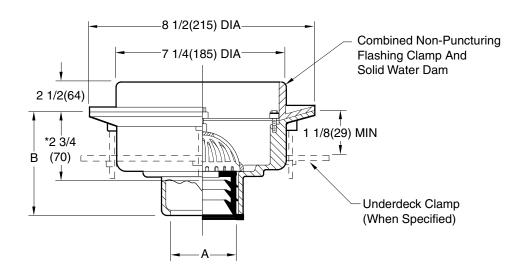
Fig. 3960C . . . CAULK OUTLET Fig. 3960Y . . . NO-HUB OUTLET
