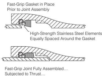
Proof-of-design tests have confirmed that the joints are capable of restraining dead-end thrust of two or more times the rated working pressure, as applicable. These tests
