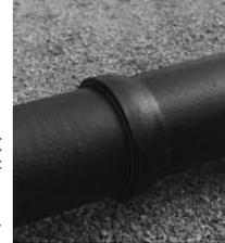
If the joint is to be deflected less than 2 1/4° for 20", 1 3/4° for 24", and 1° for 30", simply push the pipe spigot until it contacts the back of the socket and deflect. If the joint is to be deflected greater than these amounts, push the pipe spigot into the bell (while in straight alignment) only until the leading edge of the factory-applied yellow assembly stripe is even with the face of the bell. The desired deflection up to the maximum may then be set.
