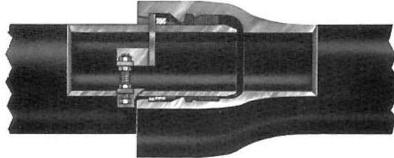
The AMERICAN Lok-Ring® Joint is another restrained joint that utilizes the sealing features of the time-proven AMERICAN Fastite Joint. It is an essentially boltless, flexible restrained connection that provides an easily assembled positive restraint against endwise separation due to thrust resulting from internal pressure or external forces. Only a minimal amount of time is required to complete the Lok-Ring assembly, or disassembly if necessary.
