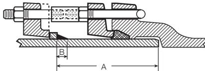
**Note:** Sizes 30"-48" use rectangular cross-section spigot glands in lieu of ductile MJ gland shown above.
