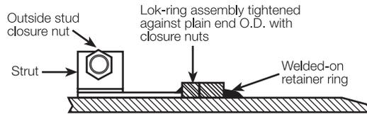
**Lok-Ring in Position for Joint Assembly**
