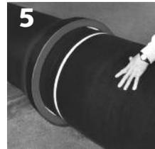
assembly procedures.) When the weld bead is in proper assembled position fully beyond the yellow Flex-Ring segments, every segment will be trapped firmly between the weld bead, the spigot, and the wedging surface of the socket.
