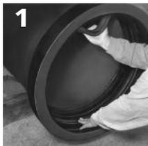
**1). Important: A Fastite gasket must also be used, because the rubber-backed flex-ring does not perform any sealing function.**
