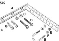
Mark position for lag screws so that square channel is located next to the pipe closest to Shut-Off Valve. Screw "C" channel into wall stud with Lag Screws. If no stud is available, use the A10 Alligator™ Anchors by following their instructions below.
