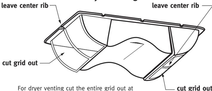
For dryer venting cut the entire grid out at both ends. Leave the center rib. Use tin snips to cut grid out before installing hood to soffit.
