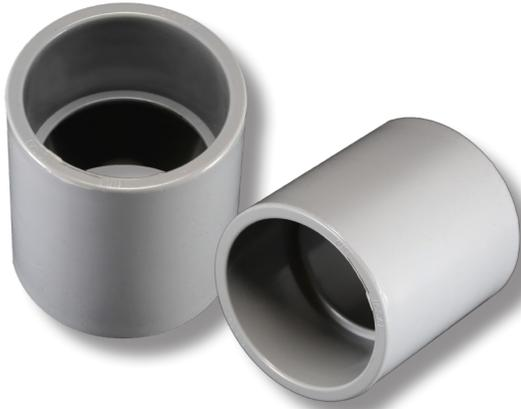
Schedule 40 Standard Center Stop Couplings are used to join lengths of conduit pipe together with two solvent weld socket ends.
