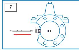
Step 7: Remove tool from Threaded Swivel Insert
