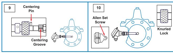
Step 9: Line-Up Centering Groove on straight threads with Centering Pin; push to seat o-ring
