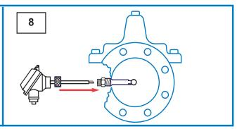
Step 8: Insert tip of e-FlowMeter Sensor/Head Assembly into Threaded Swivel Insert
