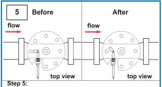
• Once inserted into the Threaded Swivel Insert tube, the Installation Tool will engage the top face of the Measurement Cylinder and force it to the 45° position, as shown above
