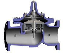
6. Caution must be taken in the installation of this valve to insure that galvanic and/or electrolytic action does not take place. The proper use of dielectric fittings and gaskets are required in all systems using dissimilar metals.
