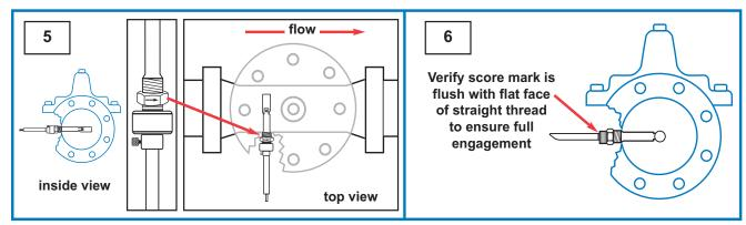
**Step 5:** Insert straightened Swivel Insert/Measurement Cylinder Assembly into valve, orient arrow on wrench flat to point downstream
