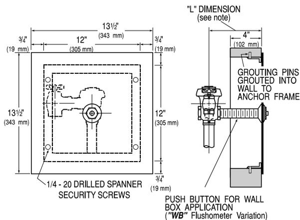
**NOTE:** "L" Dimension is the Wall Thickness (to the nearest whole inch) plus 2¾". Specify "L" Dimension when ordering Flushometer.
