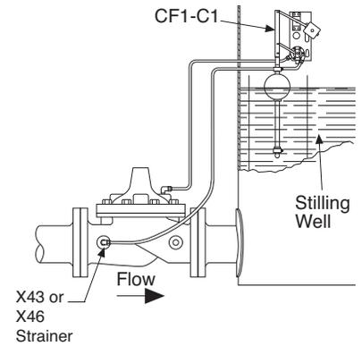
Note: We recommend protecting Float Control tubing and valve from freezing temperatures.
