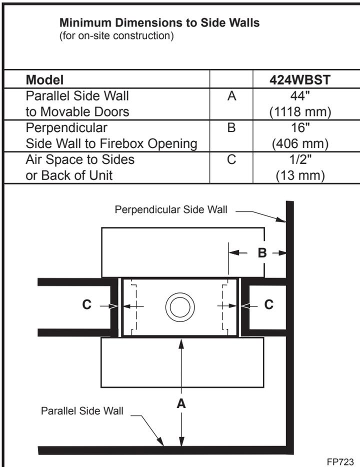
Fig. 23 Minimum firebox dimensions from combustible materials.
