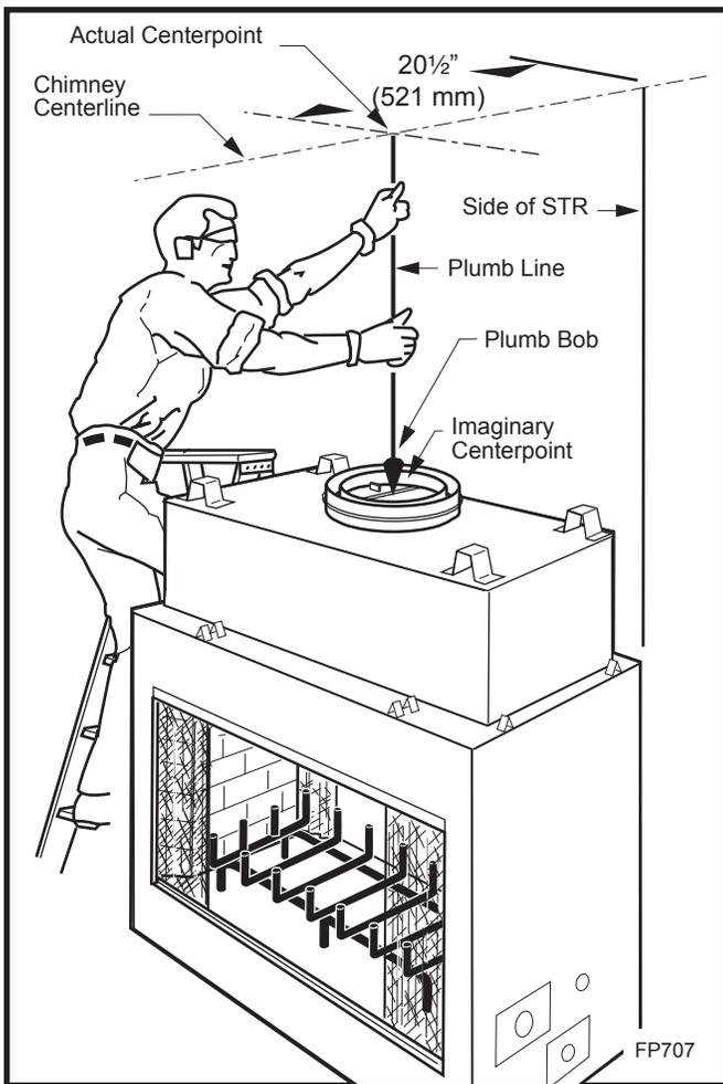
Fig. 10 Locate centerline of chimney with plumb line.
