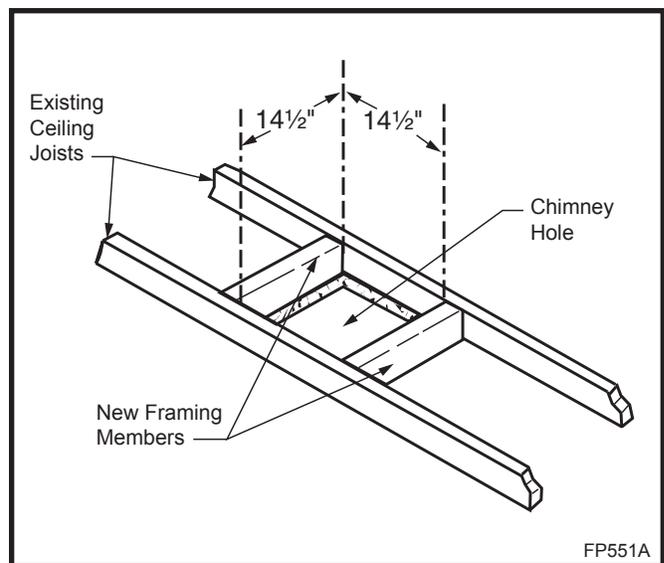
Fig. 12 Typical frame for ceiling chimney hole.
