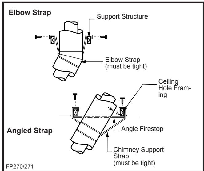
Fig. 17 Attach straps to a structural framing member.
