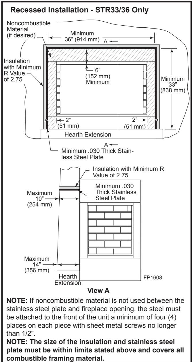
Fig. 28 Recessed installation.
