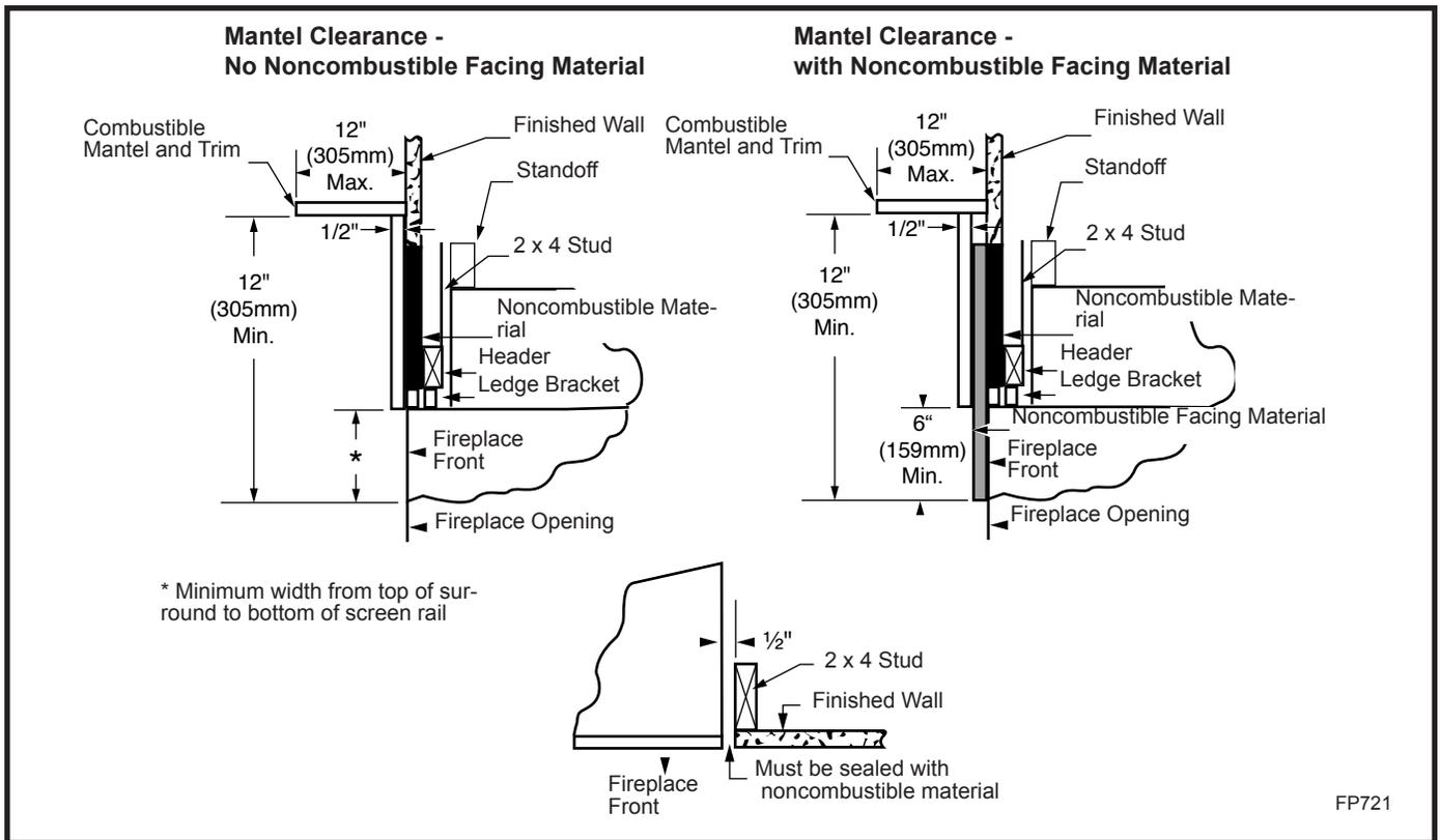
Fig. 21 Fireplace surround flush with finished wall.
