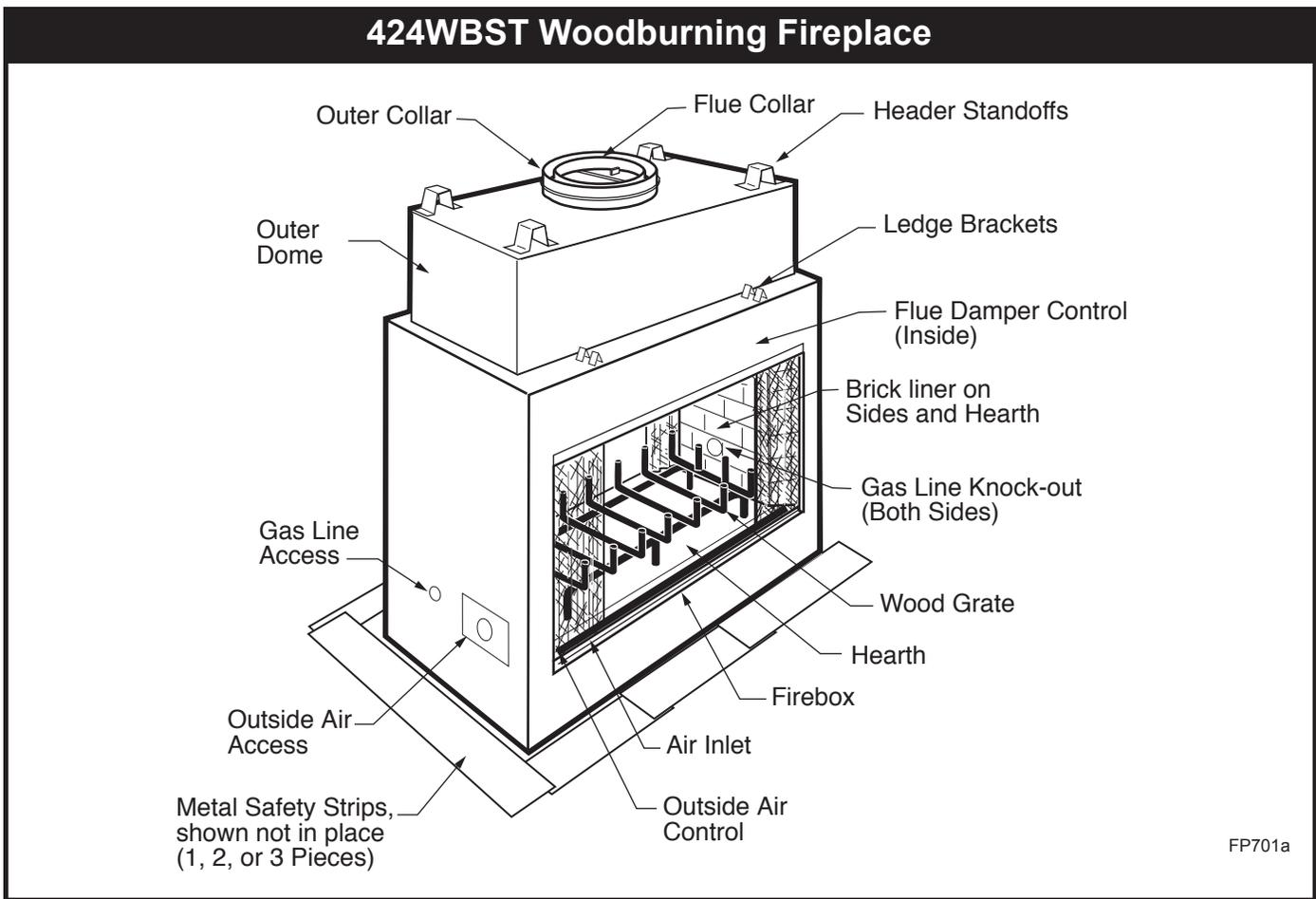
Fig. 3 424WBST Parts Identification.
