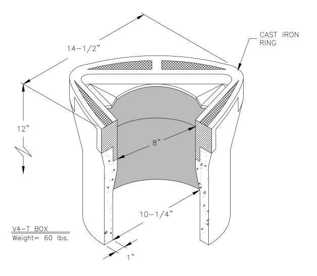
No. V4-T VALVE BOX SERIES FOR H-10 LOADING
