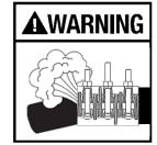
THIS PRODUCT DOES NOT RESTRAIN PIPE MOVEMENT. Proper anchoring is required to prevent pipe pull out. Failure to anchor or improper anchoring can result in dangerous pipe content escape, property damage, serious injury, or death. Refer to smith-blair.com for products designed to restrain axial pipe movement. Read the product installation instructions prior to installing this product.
