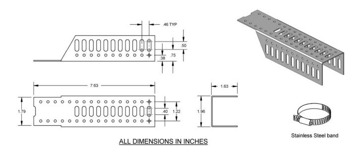
The HOLDRITE<sup>®</sup> #115 and #115-C (Copper-Bonded™) are steel brackets designed to position water supply lines off the vent or waste pipe in chase walls. Supports ½" through 2" pipes both vertically and horizontally. Packaged with self-locking stainless steel band, screws, metal clamps, and self-adhesive isolating felt. Excellent for pre-fab applications. Supports piping prior to wall framing. Heat the pipe, not the bracket when soldering the #115-C version.
