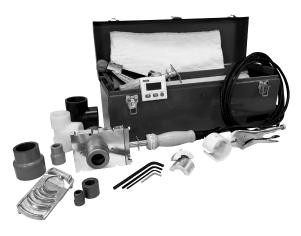
Each kit contains all of the components required for joining all sizes of socket fusion connections specified for that kit, including: heating tool, male and female heat face sets with bolts, depth gages, cold ring pipe clamp with inserts, pipe cutter, beveling tool, timer, thermal blanket, auxiliary handle, hex key wrenches, thermostat adjustment tool, joining instructions and rugged heavy duty tool box.
