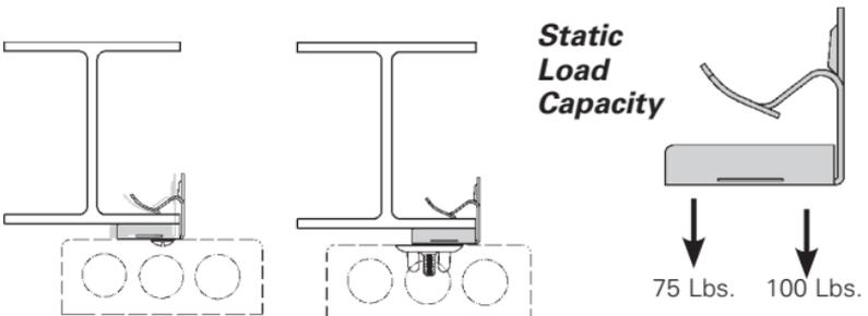
Note: Indicated loads are static load capacity and should not be combined.
