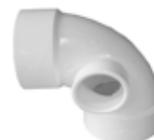
Used to connect a branch line or vent at a change of direction in a larger vertical or horizontal pipe. The inlet is constructed to accept a 2" fitting over its outside diameter or 1½" pipe into its inside diameter.
