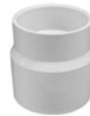
This fitting adapts Genova Sch. 40 pipe to 4" cast iron spigot and can be joined to cast iron with oakum and poured lead or poured lead substitute.
