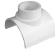
Solvent welds directly to side of sewer pipe to provide a simple way of connecting a branch into a drain pipe. The inlet is constructed to accept a 2" fitting over its outside diameter or a 1 1/2" pipe into its inside diameter.
