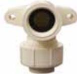
Mechanically joins 1/2" water supply piping to male pipe threads. A special elastomeric gasket ensures a leakproof seal. Usually used for a shower arm connection. Hand tighten only! This fitting seals by means of a gasket and the use of joint compound or PTFE thread tape is not necessary or recommended.
