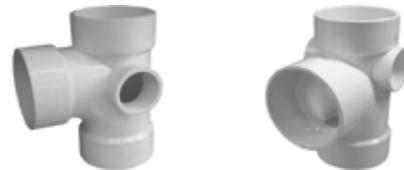
Connect 1½" or 2" vent or branch waste piping to a vertical drain pipe and receive discharge of a water closet. \*Inlets constructed to accept 2" fitting hub over outside diameter or a 1½" pipe into their inside diameter.
