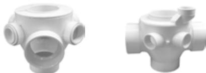
Provides for the hookup of all drains from two complete bathrooms located back to back. Each unit furnished with two flush branch plugs to enable utilizing the fitting in a left or right hand drain situation. Branch inlets are 2" socket configurations to accept 2" pipe. Bushing (Part #70221) are provided to accommodate 1 1/2" pipe.
