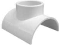
Solvent welds directly onto the side of a 3" pipe to provide a simple way of connecting a branch into a drain pipe. The inlet is constructed to accept a 2" fitting over its outside diameter or a 1½" pipe into its inside diameter.
