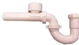
Combines the NovaVent™ anti-siphon valve and P-trap into a compact single unit. The anti-siphon trap provides a simple way of solving waste pipe drainage problems caused by inadequate plumbing system venting. Replaces almost any current fixture trap.
