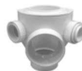
Provides for the hookup and venting of a complete bathroom. Each unit furnished with flush branch plug to enable using the fitting in a right or left hand drain situation. Branch inlets are 2" socket configurations to accept 2" pipe. Bushings (Part #70221) are provided to accommodate 1½" pipe.
