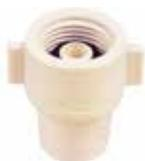
Allows a direct connection between CPVC tubing and male running threads on faucet. Has a cone washer inside female end to achieve seal.
