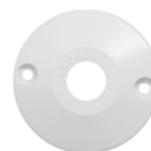
This special flange is designed to prevent torque change on CPVC pipes exiting through walls to which valves or threaded transition fittings are attached. The "torque flange" is welded to the pipe and fastened to the wall with screws thereby preventing twisting motion being transmitted to concealed joints.
