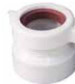
Utilized to adapt PVC pipe to tubular traps at wall or floor. Utilizes special washer which seals to either 1½" or 1¼" tubular products, reducing the number of SKU's needed in inventory. This fitting solvent welds over a 1½" DWV pipe. Sometimes called a Marvel.
