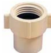
Used to adapt male hose threads to CPVC. This fitting seals by means of a gasket and the use of joint compound or PTFE thread tape is neither necessary nor recommended.
