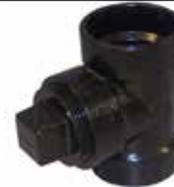
Used at the base of a vertical drain pipe to provide a cleanout opening flush with the finished wall. PTFE thread tape is recommended for threaded joints.
