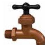
For use with female threaded fitting pipe in cold or hot water up to 150 PSI @ 180°F. (3/4" hose thread) Do not use other material compounds unless approved by the manufacturer. PTFE thread tape is recommended for threaded joints.
