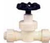
The unique valve mechanically joins water supply tubing utilizing a special locking ring and elastomeric seal. It can be used to join PEX, copper or CPVC tubing.
