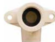
This elbow adapts from 1/2" CPVC to 1/2" male metal pipe threads and features lugs for fastening. A special elastomeric gasket ensures a leakproof seal. Used on tub and shower faucets to adapt from the 1/2" CPVC riser to the chrome shower arm. Sometimes called a "Drop Ear" elbow. Hand tighten only! This fitting seals by means of a gasket and the use of joint compound or PTFE thread tape is not necessary or recommended.
