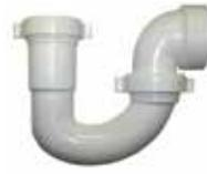
Adaptable 1 1/2" x 1 1/4" washer included. Can be utilized to connect 1 1/2" tubes, 1 1/4" tubes, as well as adapt from 1 1/2" to 1 1/4" tubes. Furnished with special PVC elbow to allow solvent welding directly to 1 1/2" Sch. 40 pipe.
