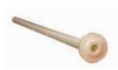
A direct replacement for flexible copper risers. Easily installed, they can be cut with a knife and are virtually impossible to kink. Can be utilized with standard 3/8" brass compression, flare fittings or patented GenoGrip adapters. Ferrule included on each tube for use with metal compression fittings.
