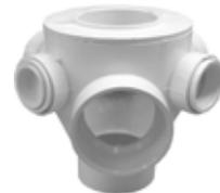
This special stack fitting provides for the hookup and venting of all drains from two complete bathrooms located back to back. Each unit includes two flush branch plugs to enable utilizing the fitting in a right or left hand drain situation. Branch inlets are 2" socket configurations to accept 2" pipe. Bushings (Part #70221) are provided to accommodate 1½" pipe.
