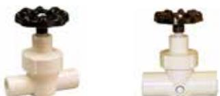
This unique valve employs the globe valve principle and is manufactured of high temperature thermoplastics. It is designed to solvent weld to CPVC tubing. This valve employs "Street/Socket" feature which allows it to be used with 1/2", 3/4", and 1" CPVC tubing. (2 - 3/4" couplings are required to attach the valve to 3/4" CPVC tubing. 2 - 1" couplings are required to attach the valve to 1" CPVC tubing).
