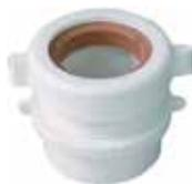
Adapts PVC fitting hub to tubular traps at wall or floor. Utilizes special washer which seals to either 1½" or 1¼" tubular products, reducing the number of SKU's needed in inventory. This fitting solvent welds into a 1½" DWV fitting hub. Sometimes called a Marvel.
