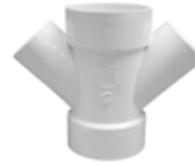
Used to bring two branch lines into a horizontal drain pipe. Branch inlets are 2" socket configuration to accept 2" pipe. The inlet is constructed to accept a 2" fitting over its outside diameter or a 1½" pipe into its inside diameter.
