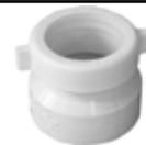
Adaptable 1½" x 1¼" washer included. Can be utilized to connect 1½" tubes, 1¼" tubes, as well as adapt from 1½" to 1¼" tubes. Solvent welds to 1½" Sch.40 drain pipe and connects via slip jamnut to either 1½" or 1¼" tubular traps. Eliminates the need for stocking extra trap adapter configurations.
