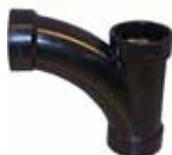
Used in some plumbing code areas to connect a branch line into a vertical drain pipe instead of a conventional tee fitting. Also, is the acceptable method of connecting a horizontal branch pipe approaching a horizontal drain pipe on the perpendicular.
