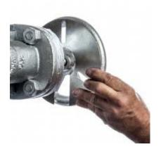
3. Follow step 2 to loosely secure the 2 remaining bolts, washers (if included), and nuts.
