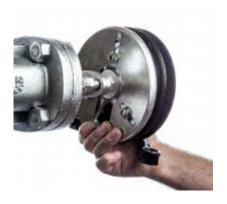
2. Place the chainwheel against the front of the valve hand wheel aligning the slots of the chainwheel to the holes in the plate. Put one washer (if included) on a bolt, pass the bolt through the top slot (12 o'clock) in the chainwheel from the front, and through the holes in the plate. Loosely secure with a washer (if included) and nut.
