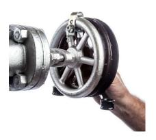
3. Follow step 2 to loosely secure the 2 remaining U straps, bolts, washers (if included), and nuts.
