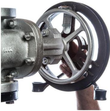
3. Put a washer (if included) on a bolt, pass the bolt through the slot in the chainwheel from the front, pass through both sides of the strap, and fasten loosely with a lock washer (if included) and nut. Repeat to fasten the remaining U strap.
