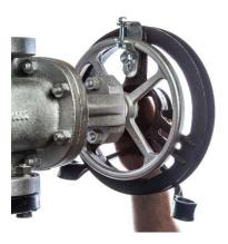
3. Follow steps 1 and 2 to loosely secure the 2 remaining adjustable clamps at 4 and 8 o'clock.
