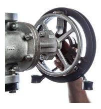
2. Fasten the adjustable clamp to valve hand wheel using the short L strap, a bolt, and a nut. Pass the bolt from step 1 through the short L strap and fasten with a nut.
