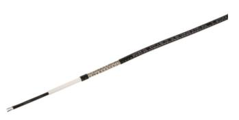
nVent RAYCHEM ETL self-regulating trace heating cables provide energy efficient pipe freeze protection. R-ETL-A/B are suitable for on- or in-pipe applications, R-ETL(-A/B)-CR for on-pipe only. Each are available in two power outputs (10 and 16 W/m at 5 °C), supported by a full range of heat shrinkable connections and accessories.
