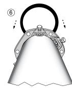
**Step 6** • Stretch gasket over pipe with beveled edge toward the bell.
