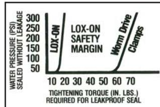
Performance graph shows sealing results of all stainless Lox-On compared to average of four brands of all stainless worm drive clamps on 1" polyethylene pipe over a 0.985" smooth plug.
