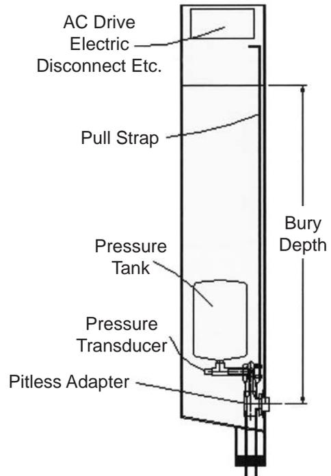
PCM for Variable Speed Pump Steel or PVC Casing
