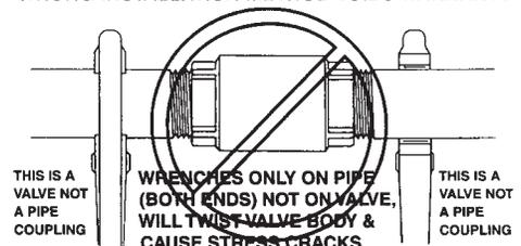
**NOTE:** All Merrill check valves and foot valves, water, oil or gas, working pressure 200 PSI, maximum operating temperature 190° F (87° C).
