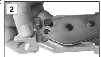
Make sure the jaws form a "V" when installed.
