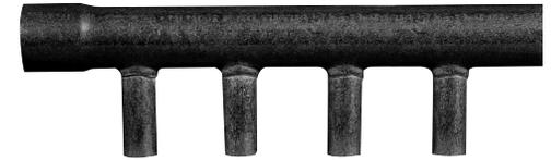
One end of the manifold body is flared to accept 1-inch fitting adapters. The other manifold end is 1" copper pipe size and requires a copper end cap, coupling or transition fitting to make the proper connection. Do not exceed acceptable flow rates for 1-inch nominal copper.
