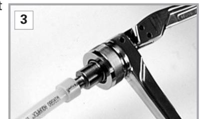
When using the ProPEX Air or Battery Expander tools, slide the expander head into the tubing until it stops. Full expansions are necessary to make a proper connection. Press the trigger to expand. Release the trigger, remove the head from the tubing and rotate it  $\frac{1}{8}$  turn after each expansion. Slide the tool head into the tubing in the newly rotated position and expand again.
