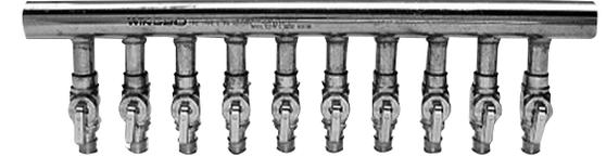
Both 1-inch ends are copper pipe size, and require a copper end cap, coupling or transition fitting to make the proper connection. Sections can sweat together to extend the number of valved outlets using a standard 1-inch copper coupling. Do not exceed acceptable flow rates for 1-inch nominal copper.
