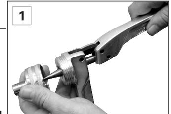
2. Select and prepare the proper APR Ratchet Tool, red (1/2- and 3/4- inch) or black (all sizes). To change jaws on the APR Ratchet Tool, open the handles slightly to relieve pressure against the jaws. Push the retaining pin back and pull the head of the pin away from the tool.
