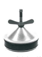
The Series A Wing Nut Test Plugs are designed and developed for testing for leaks and for sealing off sections of pipelines generally made of cast iron, steel, vitrified clay, concrete etc. These plugs come with a hollow stem which can be used as a fill or drain pipe. Turning the wing nut expands the rubber ring tightly against the inside of the pipe. Hand tightening is usually adequate in smaller sizes, but a wrench can be used on larger sizes to give a better seal.
