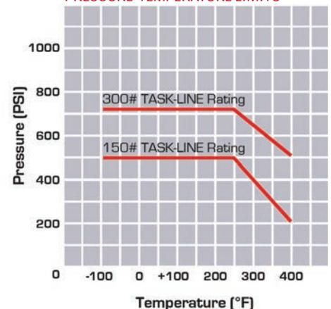
Task-Line gaskets have been tested in excess of the above pressures. Consult factory for higher pressure applications.
