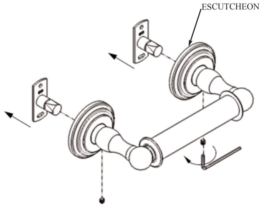
② ALIGN MOUNTING BRACKETS AND MARK LOCATION
