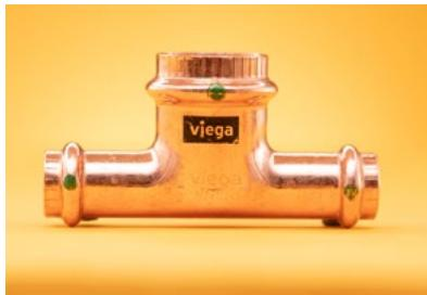
Viega ProPress may only be pressed onto copper tube in accordance with ASTM B88 or B75. When pressing onto B88 copper tube, types K, L, and M may be used. Tempers O60 and O50, known as "soft copper", are limited to nominal sizes  $\frac{1}{2}$ " to  $1\frac{1}{4}$ ". Temper H58, known as "hard copper", may be used with nominal sizes  $\frac{1}{2}$ " to 4".
