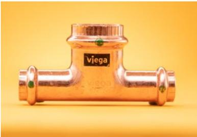
Viega ProPress may only be pressed onto copper tube in accordance with ASTM B88 or B75. When pressing onto B88 copper tube, types K, L, and M may be used. Tempers O60 and O50, known as “soft copper”, are limited to nominal sizes ½" to 1¼". Temper H58, known as “hard copper”, may be used with nominal sizes ½" to 4".
