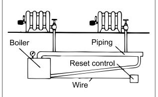
Boiler/Steam supply must be cycled by a reset control and must not run at constant pressure (which would prevent air from entering back into the system).
