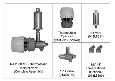
When the setting temperature is reached, the 1PS valve will be closed and no further air venting takes place.
