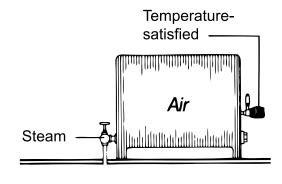
To aid in preventing overheating of rooms that are temperature satisfied, boiler steam pressure must be kept low, recommended normally at or below 2 psig. Otherwise air will be compressed in the radiator, allowing steam to enter when not required.
