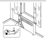
Available for mounting the 1PS assembly onto convectors are 1/8" 45° street elbows, part number 013L8300. When ordering these elbows two pieces are needed per convector.
