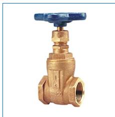
**Specifications UPC** Code 039923614179 Gate Valve Type **Valve Size** 1 1/4 in BRZ Cast Bronze Material Description T113 11/4 THD 125# NRS GATE BRZ Multi-Turn **Turns / Operation** Seat / Seal Material **Bronze Connection Type** T -- Female NPT Thread (FIPT) Valve Gate Stem Design NRS - Non-Rising Stem Valve Multi-Turn Bonnet Design Screw-in Bonnet Standard Handwheel **Operation Type**
