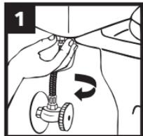
**1. Turn off water supply. Flush toilet & remove excess water from tank. Disconnect water supply connector from fill valve.**
