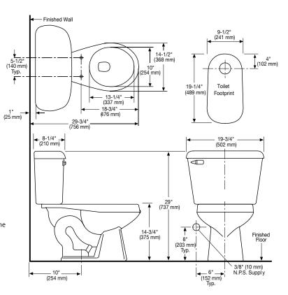
NOTE: Install this product according to the installation guide. Fixture dimensions are nominal and conform to tolerances in ASME Standard A112.19.2
