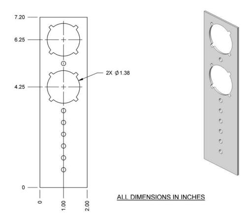
The PEXRITE® #709 is a 14 gage galvanized steel bracket with 1-3/8" keyed holes providing an approximate 4" and 6" center line off of the floor surface. Designed to work with our PEXRITE® #704 insert. Ideal for lavatories, toilets and hose bibs. Compatible with HOLDRITE® #100 and #400 series inserts.
