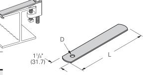
\*\* Wt./C based on 6" (152.4) length. For each additional inch in strap length add 4.2 Lbs (1.9 kg) to Wt./C.
