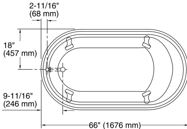
No change in measurements if connected with drain illustrated. (K-7178)
