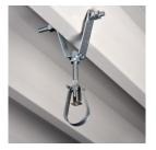
The 115 Standard Duty Loop Hanger is ideal for suspending stationary, non-insulated pipe lines, including CPVC pipes, in fire sprinkler systems. A knurled insert nut helps simplify vertical adjustments and flared edges on the base (1/2" to 4" sizes) help protect pipes from coming into contact with any sharp edges of the hanger.
