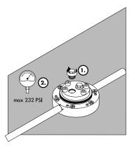
Make all water connections. Remove the two nylon plugs from the top of the white nylon test cover on the brass rough-in flange, and screw hose bibbs into the threaded openings. Pressurize the piping system and check for leaks. Attach a hose to the hose bibbs and thoroughly flush the hot and cold piping of all debris.
