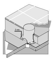
• Finish flooring can now be completed. The outside surface of the finished floor MUST fall somewhere between the "minimum" and "maximum" markings on the shield. Rough-in is now complete.
