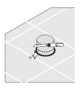
Remove the four hex-head screws that secure the white nylon test cover to the brass rough-in flange. Put the screws in a safe place - they will be re-used. Lift the test cover off. The test cover may be discarded. Make sure not to allow any debris to fall onto the brass rough-in flange.
