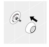
Push the spray face firmly over the spray body. Secure in place with the white c-clip.
