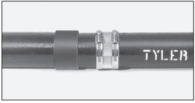
2. Insert spigots into sleeve. Be sure that both spigots butt on center retainer inside sleeve.
