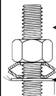
Smith-Blair® Belleville washers (p/n 150115-000) must be used on PE pipe installations. Use of any other type of spring washer may cause product failure. Do not remove flat washers.
