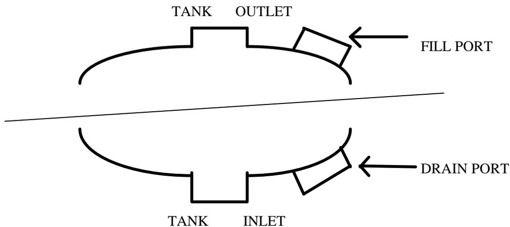
4. Once the pressure has been removed from each tank, remove the lower (drain) port plug. Desiccant will start to drop out of the 1/2” port. It is easiest to vacuum the desiccant out with a shop vac; however, the desiccant will drop out of the tower. You may have to probe the outlet with a thin probe in order to keep the desiccant from jamming together at the port. The desiccant is white in color; yellow means the desiccant has oil on it.
