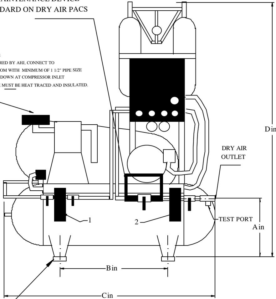
1" THICK VIBRATION ISOLATION PADS SHIPPED WITH UNIT.
