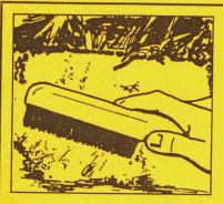
Clean application surface with wire brush. Surface must be clean, dry, and free of any loose debris. The presence of any foreign material (paint, oil, etc.) may affect adhesion.
