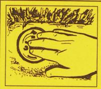
Place the marker on the application surface. Push down HARD with a twisting motion forcing adhesive out from the edge. It is important that the entire edge of the marker is sealed to the application surface.
