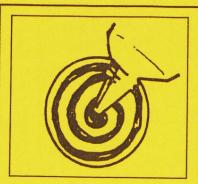
Apply adhesive to the back of the marker as shown. Start 1/6" in from the outside edge applying an even bead around the entire edge and then work to the center.
